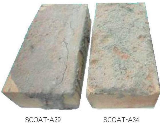
Fig.10 Adhesion status of SCOAT-A29 and SCOAT-A34 after heated in practical coke oven coking chamber for 1h.
